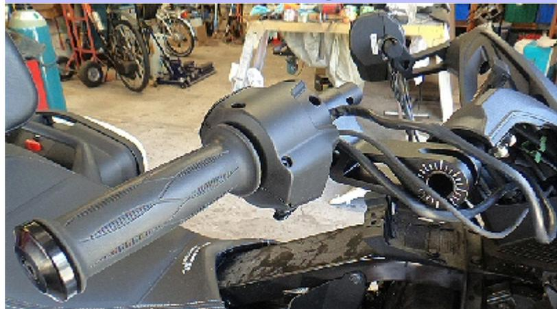
Risers on, right side wiring looms loose.
