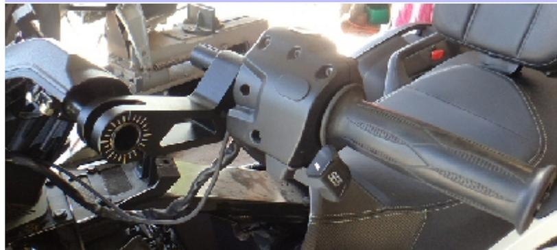
Risers on, left side wiring looms loose.
