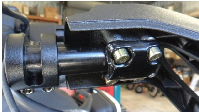
Four bolts hold the lower stub-bar securely.
