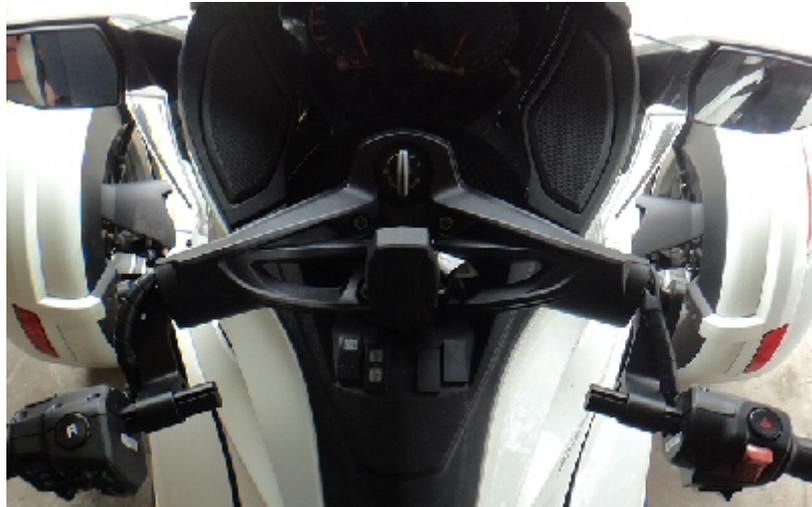
Stub-bars protruding on the inside.
